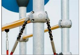
The Corocord Smart Clamps are carefully designed to ensure superior flexibility in highquality aluminum material. The smart clamps are attached around the post with four steel bolts. Unused attachment points are closed with PA caps.
