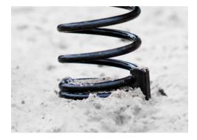
KOMPAN Springs are made of high quality spring steel according to EN10270. The springs are cleaned by phosphating before they are painted with an epoxy primer and a polyester powder coating as top finish. The springs are fixed by unique anti pinch fittings for maximum safety and long lifetime.
