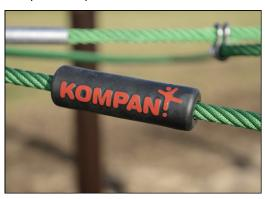
Ropes of UV-stabilised PES rope strands with inner steel cable reinforcement. The polyester yarn is made of +95% Post-consumer materials and is inductively melted onto each strand to obtain excellent wear and tear resistance.
