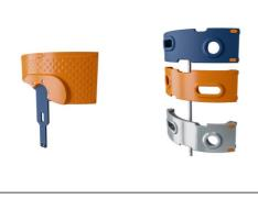
The climbing elements displayed are moulded in one piece with a minimum 5mm wall thickness. The climbing elements are made of recyclable PE, which has a high impact resistance across a wide temperature span which ensures vandal resistance.
