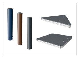
The main posts are made of high quality pregalvanized steel with powder coated top finish. Post tops are closed with caps of UV stabilized nylon (PA6). The grey colored molded decks are made of 75% post-consumer ocean waste PP material with a non-skid pattern and textured surface. All decks are supported by uniquely designed, low-carbon aluminum profiles with multiple attachment options.
