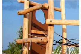
Plywood climbing panel. The climbing panels are made of 21.5mm thick plywood which comes from alder and pine wood. Both sides are covered by two layers of phenolic film with an anti-slip net pattern. All cutting edges are sealed with paint to ensure longevity.
