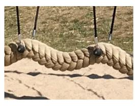
The rope of the pendulum swing is made of polypropylene (PP) rope in Coconut style with a square shape of 14x14cm. The ends of the Coconut rope are closed by a steel clamps and sealed by a glued-on shrinkable tubing. The last 10cm of the rope ends are cut open to make a tassel with bumper function to fulfill global safety requirements.
