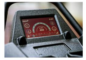
The durable 7" LCD, touchscreen with IK8 protection glass gives instant feedback on speed, distance, time, burned calories etc. The resistance of the crosstrainer can be adjusted on the screen.
