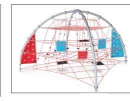
The bent arches are holding the tensioned net structure without additional disturbing fasteners. Therefore, the arches are produced from high degree stainless steel to allow movement of the net on the surface of the steel arches. The surface is then treated to create a shiny finish.
