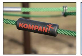
Ropes of UV-stabilized PES rope strands with inner steel cable reinforcement. The polyester yarn is made from +95% post-consumer materials and is inductively melted onto each strand. Colored steel components have a base of hot dip galvanization and a powder coated top finish. This provides an ultimate corrosion resistance in all climates around the world. Other steel surfaces are hot dip galvanized inside and outside with lead free zinc.
