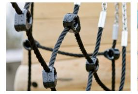
Nets and ropes are made of UV-stabilized PA with inner steel cable reinforcement. The rope is induction treated in order to create a strong connection between steel and rope which leads to good wear resistance.
