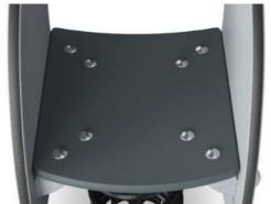
Seat is made of Ekogrip™ panel that consist of a 15mm thick PE base with 3 mm top-layer of soft rubber with a non-skid effect.
