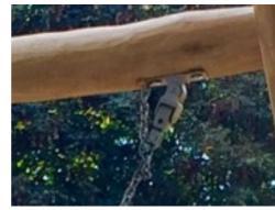
Swing hangers for Robinia wood crossbeams are made of stainless steel brackets and can move over two axis. The flange bearings are silicone enriched to make the suspension maintenance free.
