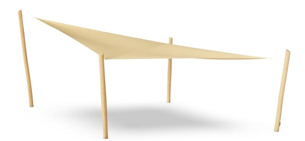
KOMPAN Robinia sunshades are designed to provide shaded play areas on sunny days. Sunshades are often used to cover areas where kids are sitting still for a longer time like for example sandboxes and playhouses. The shading is elevated by posts in each corner and the sail is attached to the post by a nylon rope and tightened in a V-track. The high-
