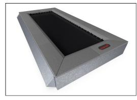
All steel components are manufactured from carbon steel S235 in a thickness of 3 mm. Side panels, support walls for top frame, plates bended with SBR and plates flat for in-situ surfacing are hot dip galvanized. The two long side panels are electro galvanized and powder coated.
