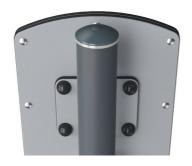
Steel posts are made of Ø101,6 x 2,0mm pregalvanized steel tube. The posts are powder coated .Tops of posts are sealed with plastic caps (PA6). Footings for surface installation are manufactured from Carbon steel with hot-dip galvanized surface according to ISO1461.
