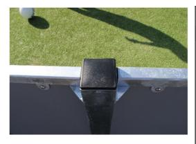
The posts are made of  $80 \times 80 \times 3$ mm profile with horizontally, 6mm welded flanges. This will enable easy installation and strong construction. The low-density polyethylene post caps are attached with blind rivets.
