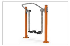
The arms for the foot pedals are 855mm long, and made from ø48,3x4mm S235JR hot dip galvanized steel tube.
