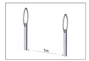
The stand can hold up to two bicycles. When place inline the recommended distance from stand to stand is 1000mm
