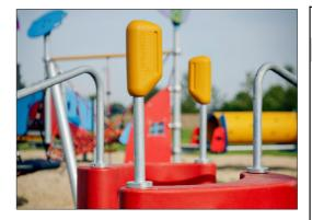
The themed post comprises 100% recyclable PE from 33% post-consumer materials. It is molded in one piece with a minimum of 4 mm wall thickness to ensure high durability in all climates worldwide.
