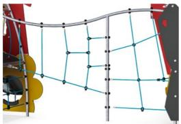
Ropes are made of UV-stabilized PP rope strands with inner steel cable reinforcement. Horizontal ropes are PUR coated to obtain good wear and tear resistance.
