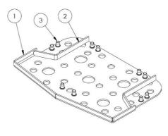
A 5 mm hot-dip galvanised carbon steel plate must is moulded inside the SBR to offer optimal stability and optimize the mounting of the step
