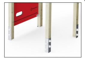
The main posts are equipped with hot-dip galvanised steel footings. The steel footings elevate the posts position 20mm from ground level to avoid contact with surfacing material.
