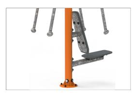
The Steel posts are made of Ø101,6x2,0mm pre-galvanised steel tube. The posts are powder coated, corrosion class C3 according to ISO12944-2.
