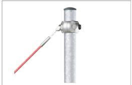
Corocord smart clamps are carefully designed in every detail to ensure superior flexibility in high quality aluminum material. The smart clamps are attached around the posts with four steel bolts. Not used attachment points are closed with PA caps.
