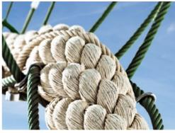
The PP rope in coconut style has a diameter of 150 mm. The internal steel wire core has thimbles at both ends, which serve as attachments for the rope to existing connecting elements.
