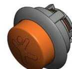
The push buttons and the housing for the push buttons are made from Polyamide (PA6). The buttons contain a magnet which activates a contactless reed switch when the buttons are pushed. This ensures high durability of the system.
