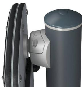
The connectors are made of die-cast aluminum specially alloyed for outdoor environments and with a lead content below 100ppm. The connectors are attached to the posts by stainless steel screws and well protected against corrosion by special designed zinc washers. Extremely strong and no change of corrosion.
