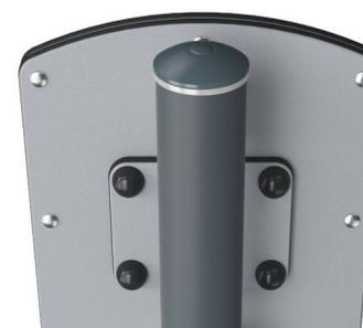
Steel posts are made of Ø101,6 x 2,0mm pre-galvanized steel tube. The posts are powder coated. Tops of posts are sealed with plastic caps (PA6). Footings for surface installation are manufactured from Carbon steel with hot-dip galvanized surface according to ISO1461.
