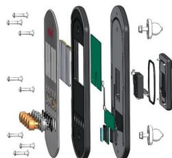
Front panels are made of UV-stabilized Polycarbonate. The UV-stabilization prevents the Transparent panels in being yellow over time and ensures the mechanical performances. The graphic prints are added by a unique multi-layer print process where the inner layer is the image and outer transparent layer functions as protection. The lacquer is water-based, and UV stabilized to prevent fading.
