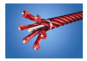
Saturn ropes has six-stranded steel wires and a steel wire core. Each strand is tightly wrapped with PES yarn, which is melted onto each individual strand. After initial friction has removed the surface fibers, a harder PES coating remains to protect each strand, making the ropes highly wear- and vandalism-resistant.
