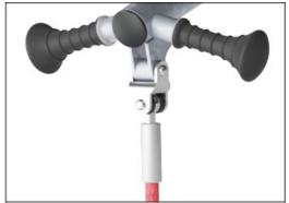
The two angled top handles are made of a molded PP insert with an outer soft layer of TPV rubber. The handle is attached to the pipe with a galvanized steel inlay to ensure strength and durability.
