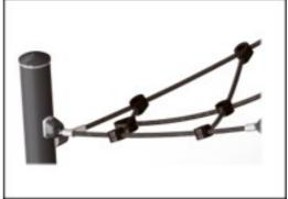
Rope loops of the seat are made of single braided 16 mm PES ropes. PES has high strength with excellent resistance to abrasion and UV radiation. The rope loops are connected by nylon (PA6) connectors.
