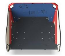
All floors are made of High Pressure Laminate HPL with a thickness 17.8mm and non skid surface texture according to EN 438-6. KOMPAN HPL has high wearing strength to ensure long lifetime in all climates.
