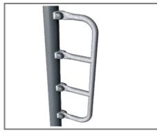
The handles offer 4 different heights to place the Post are made of Ø101.6 x 2mm, prehands or feet
