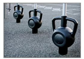
The tubes on which the magnetic bells move on are ø40mm, made of grade AW 6082-T6 aluminium and have an anodized layer of 20µm. The tube has a full steel core for structural integrity.
