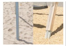
The post of the A-Frame swings is available in two mounting options; surface mounted with anchoring expansion bolts or inground in 60cm or 90cm depth. The hot-dip galvanised steel legs are anchored directly into the ground and Pinewood posts are elevated from the ground by a unique profiled hot-dip galvanised steel footing.
