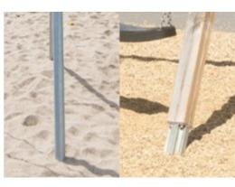
The post of the A-Frame swings is available in two mounting options; surface mounted with anchoring expansion bolts or inground in 60cm or 90cm depth. The hot-dip galvanised steel legs are anchored directly into the ground and Pinewood posts are elevated from the ground by a unique profiled hot-dip galvanised steel footina.
