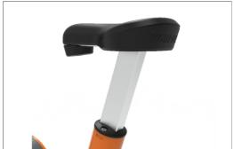
Seat is made of injection molded soft PUR with a powder coated steel inlay made from s235 steel. The user can choose between 9 different seat heights, ranging between 845mm and 995mm. The seat allows users with a height of 150cm to 195 cm to comfortably use the bike.
