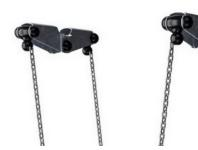
The double steel yoke suspension provides the unique parallel movement of the seat. The swing hangers are made of high quality UV stabilised nylon (PA6) housing with integrated lifetime sealed ball bearings. The height adjustable chains are fixed by a stainless steel hook with theft proof snake eye bolt in a turn able anti twist housing.
