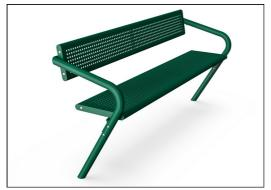
Powder coated top finish on top of galvanisation is processed in two steps: Light grinding and clean sweeping, powder coating - thickness 70-120  $\mu$ m.
