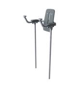
The frame of the leg lift is made from Ø38 x 2mm HDG steel tube. The support plates are made from 15mm Ekogrip®, a 15 mm PE plate with a 3 mm top-layer of thermoplastic rubber with non-skid effect. The arm supports are 110 x 195mm, 580mm apart, and 1315mm above ground. The back support is 335 x 500mm. The opening in the back is 30 x 350mm.
