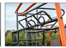
The pull up station consists of multiple handles, i.e. 2x rotating gym rings, 2x grip balls, and multiple horizontal bars at heights between 170 and 267cm with three different diameters,  $\emptyset$ 25 x 3.0mm,  $\emptyset$ 33.7 x 3.0mm and  $\emptyset$ 48.3 x 4.0mm.
