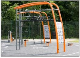
To ensure the integrity of the mainframe is maintained, the orange coloured main posts are made of  $\emptyset$ 101.6 x 3mm steel posts, which are hot-dip galvanised and powder coated in a variety of colours options. The supportive posts receive the same surface treatment and are made of  $\emptyset$ 76.1 x 3.6mm steel tubes and finished with coloured powder coating.
