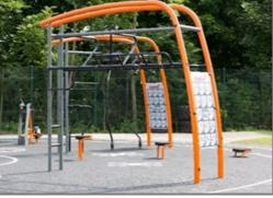
To ensure the integrity of the main frame, the orange coloured main posts are made of  $\emptyset$ 101.6 x 3mm steel posts, which are hot dip galvanised and powder coated Orange (RAL2010). The supportive posts receive the same surface treatment and are made of  $\emptyset$ 76.1 x 3.6mm steel tubes, powder coated grey (RAL7012).
