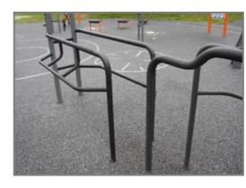
The product offers two sets of parallel bars  $\emptyset$ 48.3 x 4mm, three different heights (104, 114 and 124cm) and four lower side bars  $\emptyset$ 33.7 x 3mm. Combined these 6 bars offer a wide variety of training options.
