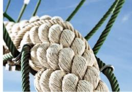
The PP rope in coconut style has a diameter of 150 mm. The internal steel wire core has thimbles at both ends, which serve as attachments for the rope to existing connecting elements.
