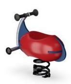
The seat is made with recycable PE from 33% post consumer materials and moulded in one piece with a minimum 5mm wall thickness. PE has high impact resistance across a wide temperature span which ensures vandal resistance in all locations.
