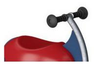
Handles are made with a moulded PP insert and an outer layer of soft TPV rubber. The handles are attached to the pipe with a galvanised steel inlay to ensure strength and durability.
