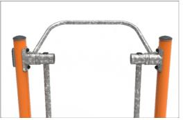
Safety bar is made of tubing with a diameter of 38 mm and wall thickness of 2 mm made of steel S235 with a hot dip galvanized surface treatment according to ISO1461 with a lead content below 90ppm for surfaces and for base material below 100ppm and with powder coated top finish.
