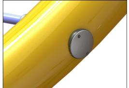
The rope is fixed to the large steel pipe by a unique KOMPAN designed tightening solution. It consists of inner and outer nylon (PA6) bushings that guides the rope to an outside threaded stainless steel part that tightens the rope.
