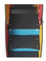
The steps are made of High Pressure Laminate HPL with a thickness 17,8mm and non skid surface texture according to EN 438-6. KOMPAN HPL has high wearing strength to ensure long lifetime in all climates.
