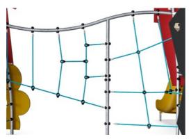
Ropes are made of UV-stabilised PA with inner steel cable reinforcement. The rope is induction treated in order to create a strong connection between steel and rope which leads to good wear resistance.
