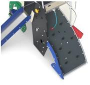
Curved climbing wall is made of Ekogrip® panel that consist of a 15mm thick PE base with 3 mm top-layer of soft rubber with a non-skid effect.
