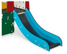
The slide bed can be chosen in different materials: Straight moulded PE or stainless steel slide bed t=2mm. Sides of the slides are made of EcoCore™. The sand strainer is made of high-quality stainless steel to ensure the durability of the product.
