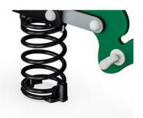
KOMPAN Springs are made of high quality spring steel according to EN10270. The springs are cleaned by phosphating before they are painted with an epoxy primer and a polyester powder coating as top finish. The springs are fixed by unique anti pinch fittings for maximum safety and long lifetime.
