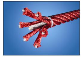
Corocord ropes with 19mm diameter or more are special 'Hercules' - type with galvanized sixstranded steel wires. Each strand is tightly wrapped with PES yarn, which is melted onto each individual strand. The ropes are highly wear-and vandalism-resistant and can be replaced at site if needed.
