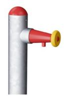
The steel surfaces are hot dip galvanised inside and outside with lead free zinc. The galvanisation has excellent corrosion resistance in outside environments and requires low maintenance. The integrated water tap open for water when pushed and stops when letting go. The water is supplied trough a pipe located inside the post with hose or pipe connection at the bottom of the post. The supply can either be a loose hose or a permanent in-ground pluming.
