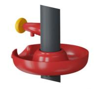
The integrated water tap open for water when pushed and stops when letting go. The water is supplied trough a pipe located inside the post with hose or pipe connection at the bottom of the post. The supply can either be a loose hose or a permanent in-ground pluming.
